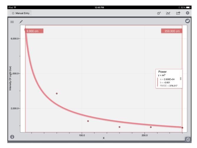
This graph shows that as the distance increases the intensity of light supplied from the lamp decreases with inverse relationship. The intensity of light equals 2.6x10^4 times distance from light to the power of -0.601
